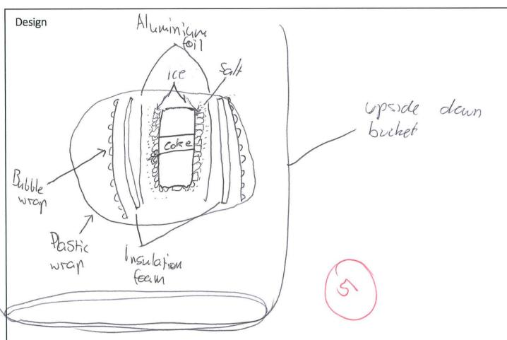
· Salt and ice react which reduces the melting point and temperature of ice. This means more heat is taken from the can to the ice because the temperature difference is higher. This is the conduction of heat.
